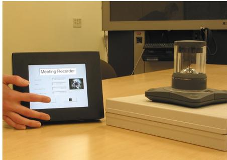
**Fig. 1** A meeting recorder prototype consisting of an omni-directional camera with 4 microphones at its base (right) and a touch-screen controlled interface on the left. The recording PC is not shown.
